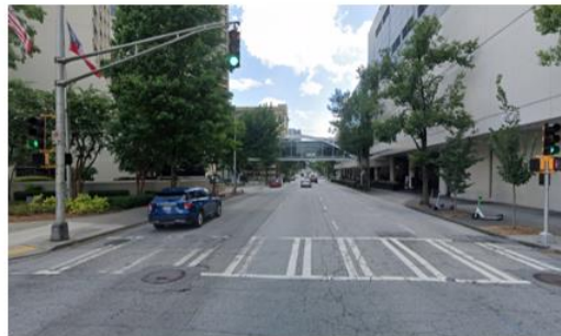
Figure 6: Supplemental Signal Heads on Pedestals in Downtown Atlanta
