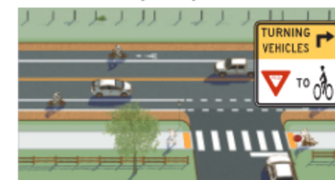
Figure 3-10. A variety of design treatments exist depending on the roadway configuration, available curb-to-curb width, traffic volumes and desire to provide a dedicated turn lane. All designs should strive to reduce speeds of turning vehicles, remind users of bicycle priority, and clarify user positioning approaching and through the intersection. Common signs at intersections include R4-4 Begin Right Turn Lane Yield to Bikes and a modified R10-15 Turning Vehicles Yield to Bikes sign. 19
