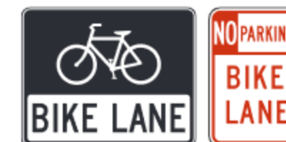
Figure 3-9. An optional R2-17 Bike Lane sign may be used to supplement bike lane markings. An R7-9 sign may be used if parked vehicles frequently block the bike lane.
