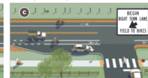
Figure 3-10. A variety of design treatments exist depending on the roadway configuration, available curb-to-curb width, traffic volumes and desire to provide a dedicated turn lane. All designs should strive to reduce speeds of turning vehicles, remind users of bicycle priority, and clarify user positioning approaching and through the intersection. Common signs at intersections include R4-4 Begin Right Turn Lane Yield to Bikes and a modified R10-15 Turning Vehicles Yield to Bikes sign. 19
