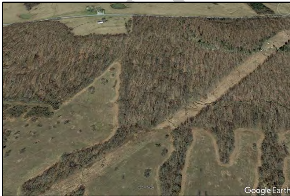
Figure 4.22. Transmission line ROW. Source: Google Earth.
